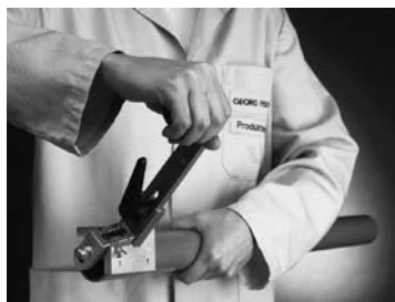
Chamfering the pipe
