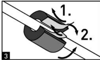
3 Assemble insulation 1. Take off foil 2. Press area of contact
